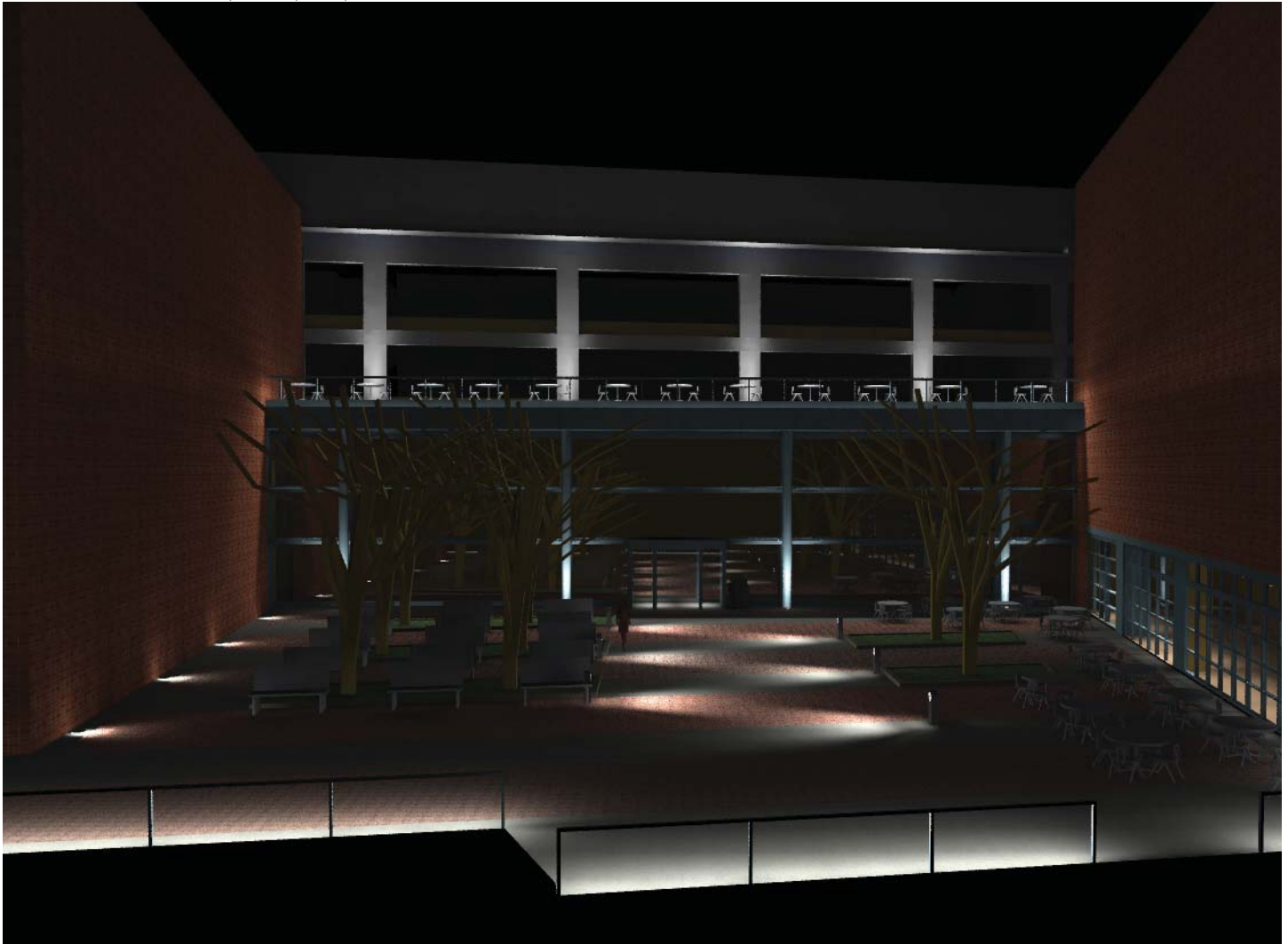
Figure A.6 – RGB raytraced rendering of terrace with new railings and redesigned lighting
