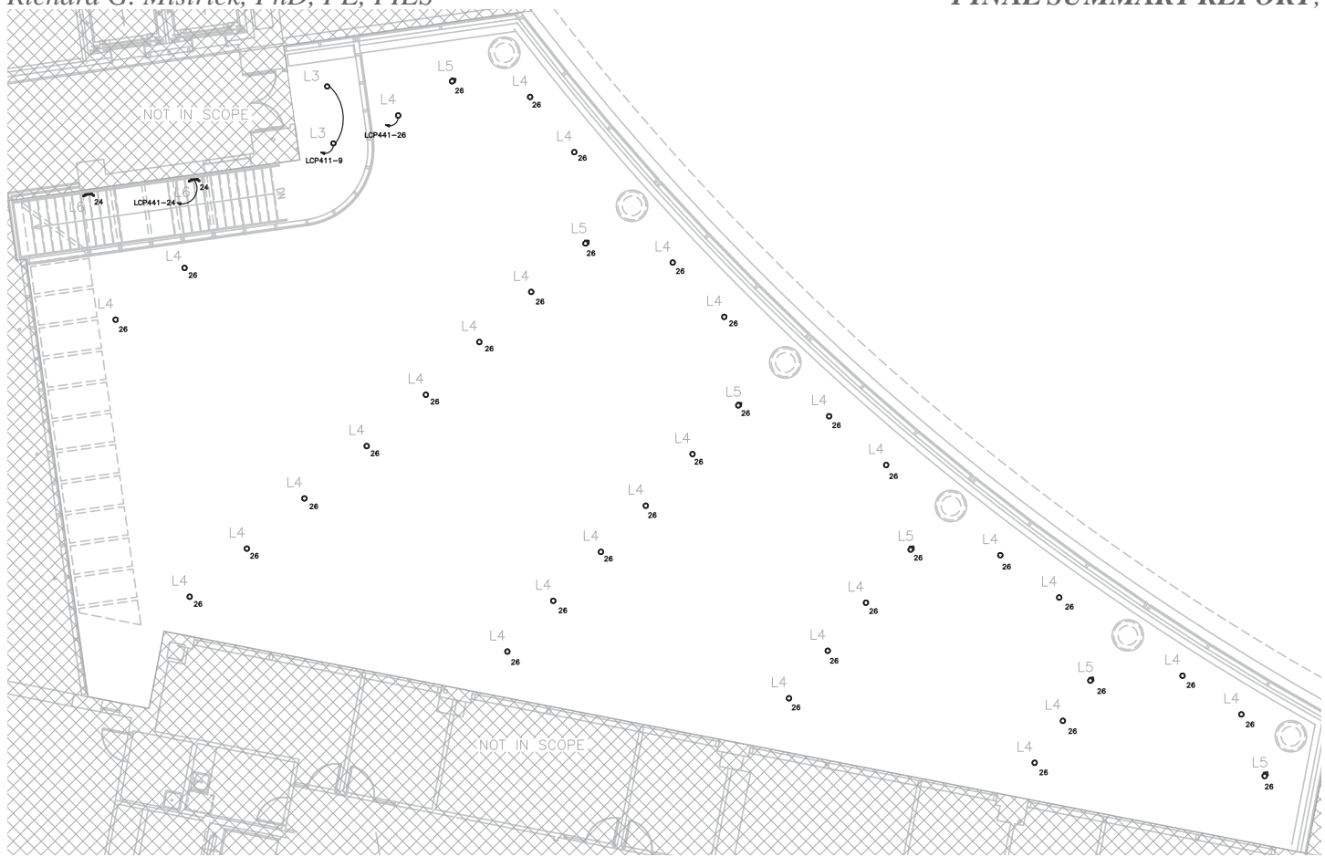
Figure B.7 – Atrium lighting plan, 4th level
